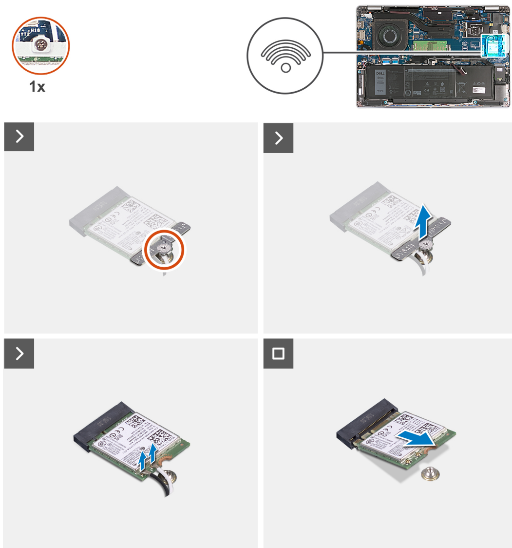
Figure 10. Removing the wireless card
