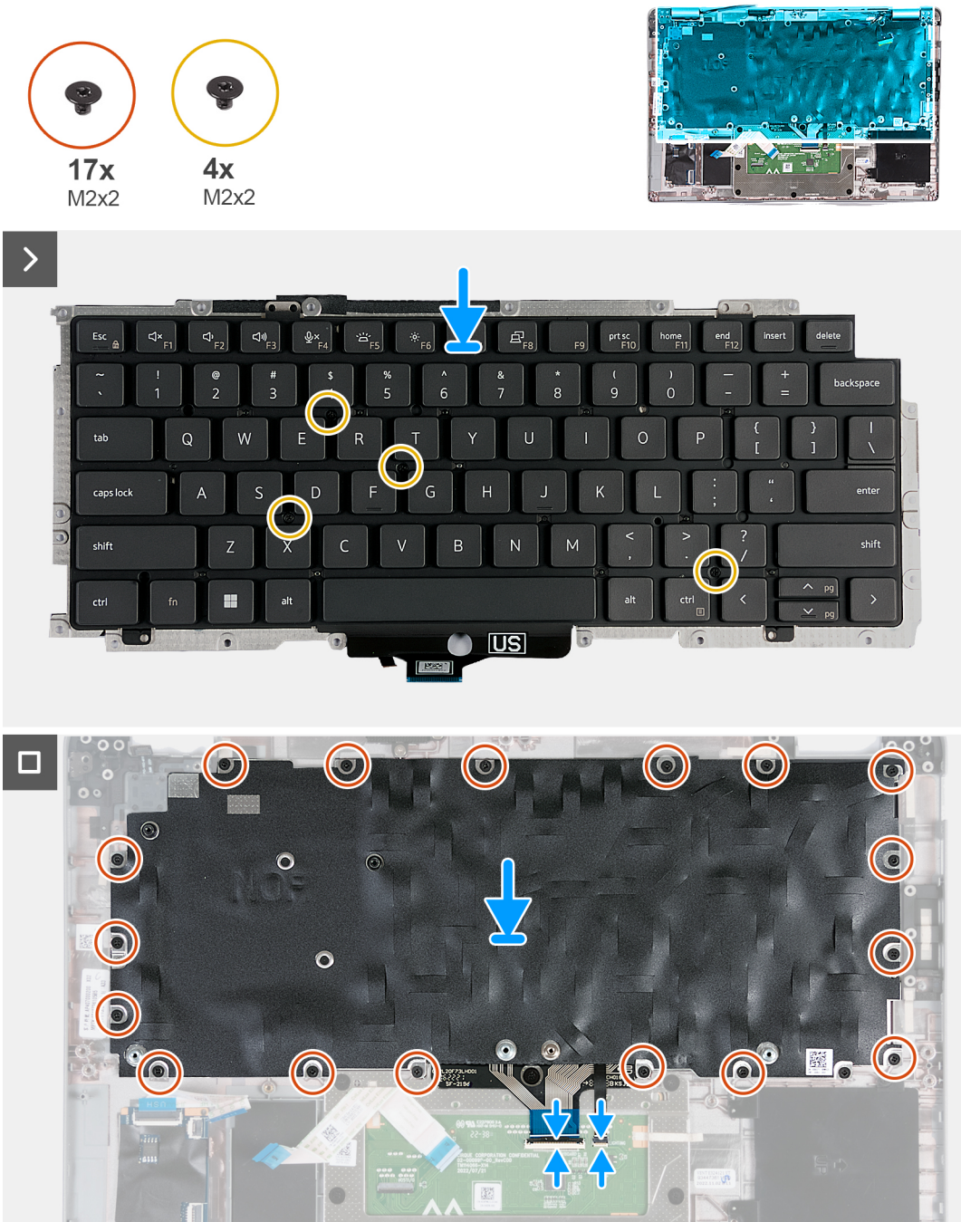
Figure 62. Installing the keyboard
