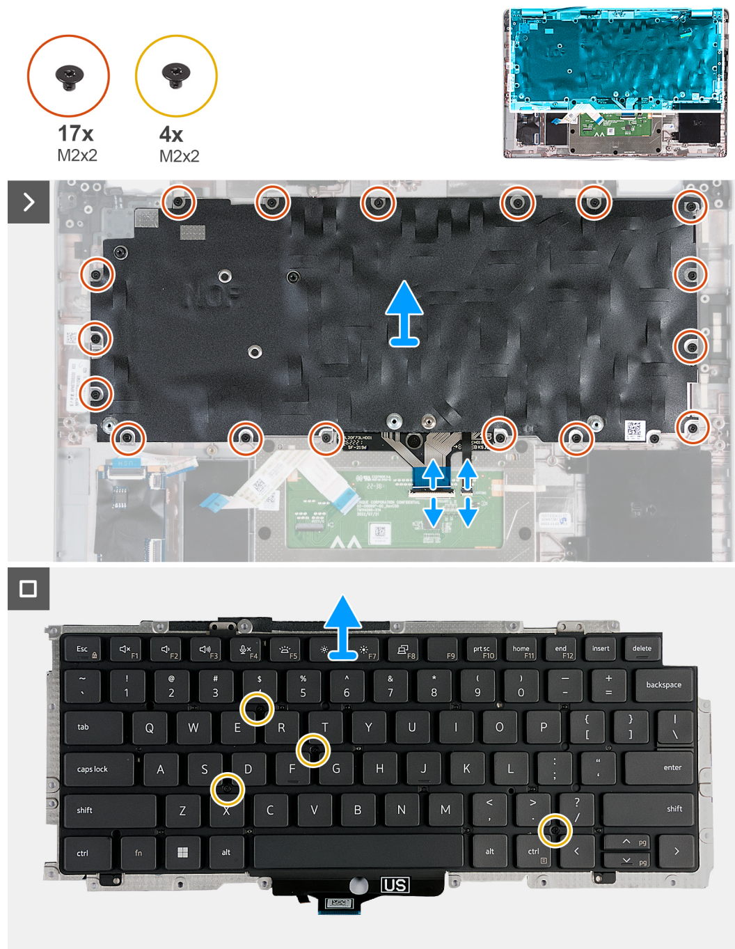
Figure 61. Removing the keyboard
