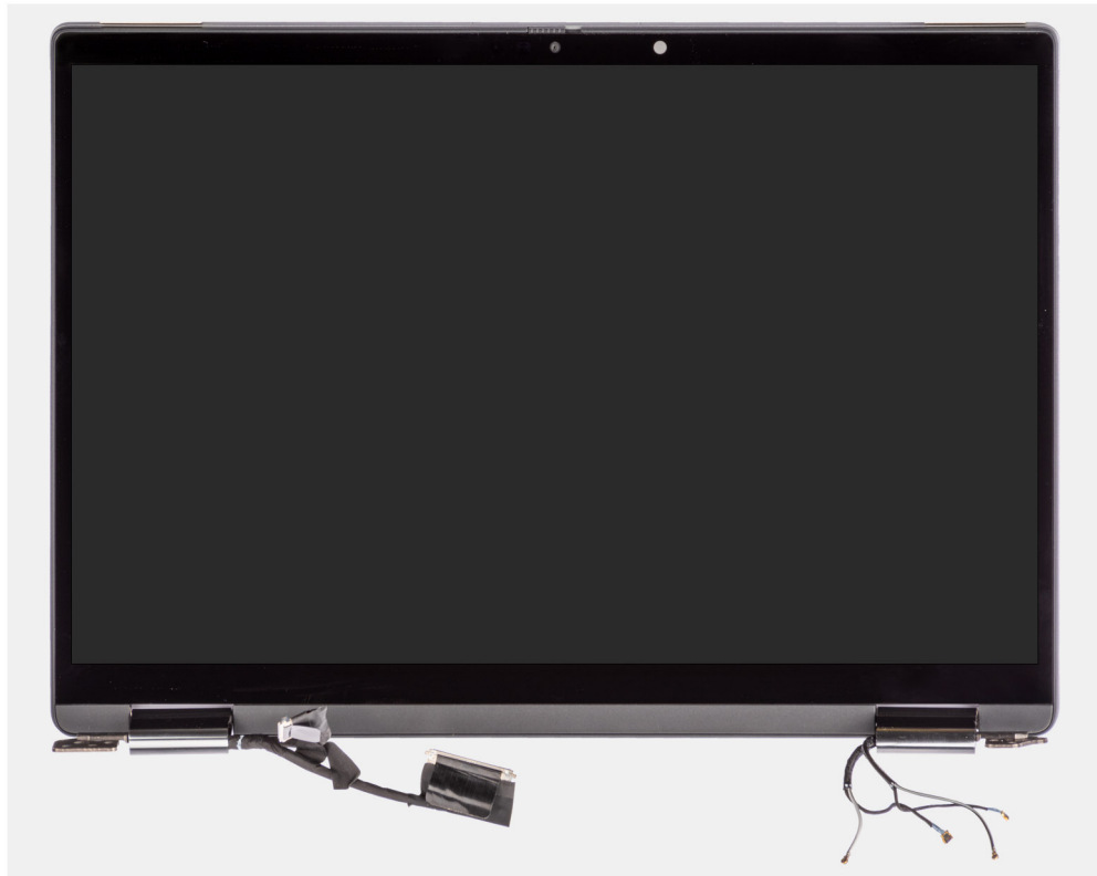
Figure 1. Display assembly without WWAN-antenna cables
